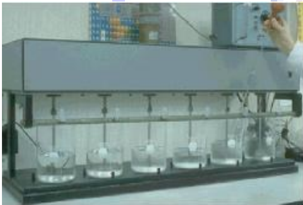
Jar Test apparatus and the expected results
